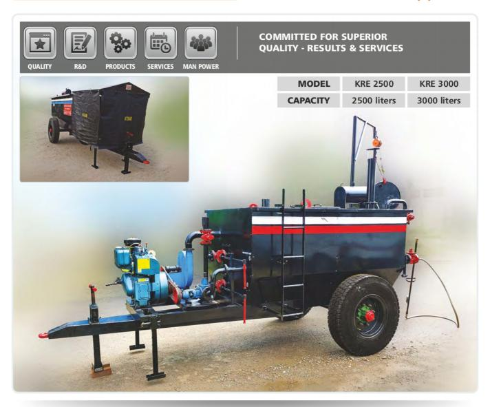
Tractor linked tyre mounted Bitumen-Emulsion Sprayer with Compressor for road dust cleaning is developed for tack / prime coat by hand spraying arrangement and intermittent spraying application with road dust cleaning also. This equipment is capable of applying uniform coating of Hot Bitumen & Emulsion on specified surface.
