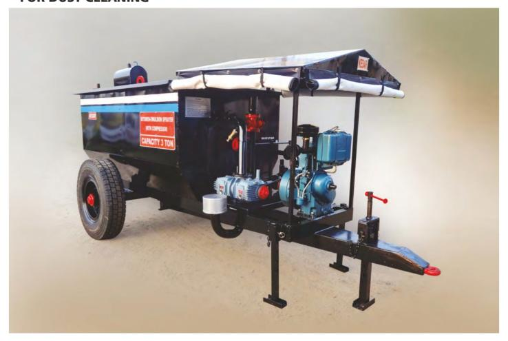
Tractor linked tyre mounted Bitumen-Emulsion Sprayer with Compressor for road dust cleaning is developed for tack / prime coat by hand spraying arrangement and intermittent spraying application with road dust cleaning also. This equipment is capable of applying uniform coating of Hot Bitumen & Emulsion on specified surface.
